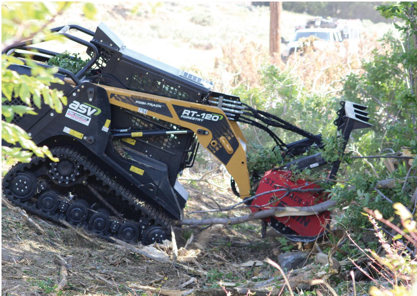
A recently purchased skid steer with a mulching head will help clear KPUD's rights-of-way and aid in fire prevention.
