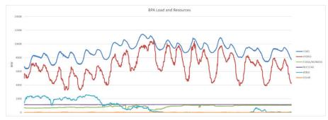
Note how the federal hydro system—the red line—flexed up and down to meet peak demand requirements. The Columbia Nuclear Generating station also cranked out power at a steady 1,200 MWs. I want to point out that wind generation supplied a significant amount of power at the start of the cold snap, then tapered off to nothing for days. Solar was nonexistent.
