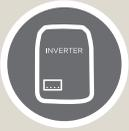
**2** An inverter, which is connected to the electric grid, converts the electricity from direct current to alternating current to make it safe for use in homes.
