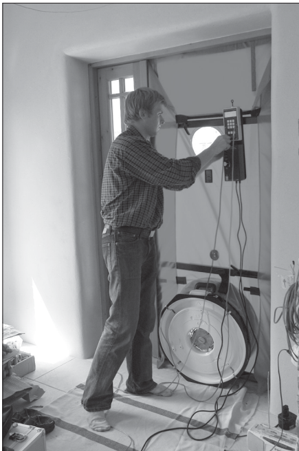
A blower door test during a home energy audit can help identify sources of air leaks.
