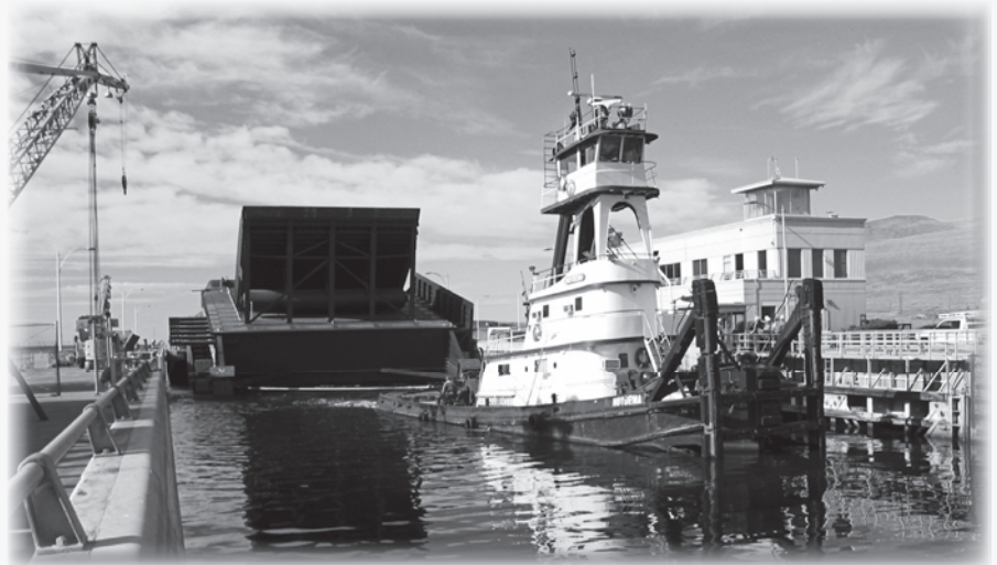
A tugboat pulls a spillway weir through the locks at McNary Dam on the Columbia River in October 2007. The weir was positioned in one of the spillways at Lower Monumental Dam on the Snake River to improve juvenile fish passage. Photo by the U.S. Army Corps of Engineers.
